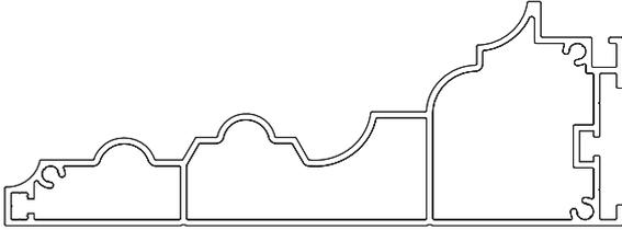
This is the profile of the frame. The frame accomodates the connection set within it's profile.
