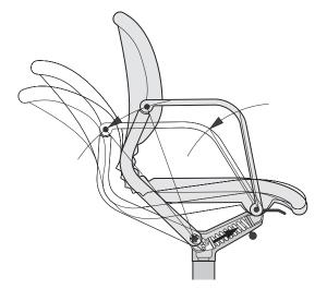
Three swivel axes are designed to allow the seat, backrest and armrests to follow any movement and change in posture.
