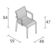
Stacking chair with arms for outdoor use with structure in stove enamelled die-cast aluminium. Seat and back in teak lists.
