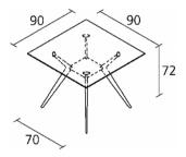
Square table with structure comprised of 4 legs in die-cast aluminium with painted or polished finishes, connected by a shelf. Top available in oak veneered plywood with solid edge, thickness 15mm, "LG HI MACS®" natural acrylic stone, thickness 15mm. Shelf available in oak veneered plywood, thickness 15mm or "LG Hi MACS®" natural acrylic stone, thickness 15mm.
