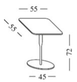
Small table with round base in stove enamelled steel finished in matt metallic grey (thickness 8 mm) and leg in stove enamelled steel finished in matt metallic grey. Maple veneered aluminium top, thickness 6 mm.
