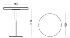
Round table with 80mm diameter stove enamelled steel leg finished in textured matt metallic grey, top in maple or in laminate and maple heart-wood edge; 530 mm diameter base in stove enamelled steel finished in matt metallic grey.
